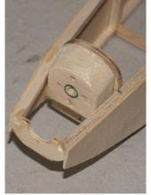
21: Now pull in the nose and glue in the bulkhead and the lower part of the front ply plate, remembering the 2 degrees right thrust. If the sides are difficult to pull in, cuts can be made in the 1/4sq stringers as before. When sides are right, drip some cyno on cuts to reinforce. Additional bits of 1/4sq were added vertically behind the bulkhead, just as a bit of strengthening.
