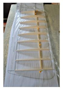
3: Roughly sand leading edge to shape. (It is easier to do this now than when fitted.) Then glue in leading and trailing edge, and top spar.
