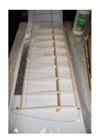
4: Fit webbing on the back of the spars, make sure that the wood grain is vertical.
