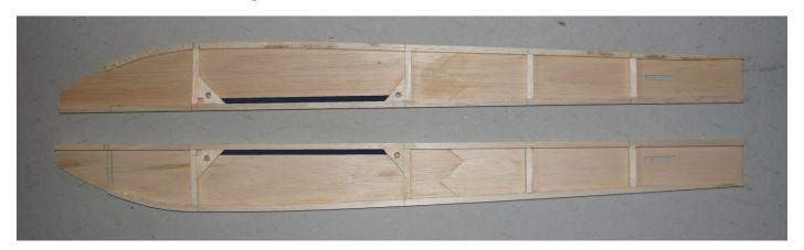
16: Again, cover plan with cling film and with the sides upside down on the plan, join together with pieces of 1/4sq at front of wing seat where the hole is in the dowel sheet. Ensuring that the sides are square.
