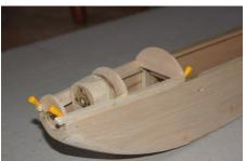
29: The front hatch is next. So pin the 1/4sq stringers in place on the fuse-lage, and fit the formers, H1, H2 and the front ply plate. When dry, the 1/16 sheet can be cut into strips and the hatch planked.
