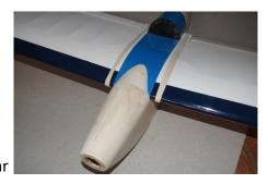
of the hatch and sand to shape. To get a good fit to the wing, I used a thin layer of P38 car body filler to get the right profile.
