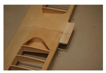
11: Bend the torque rods to the size shown on the plan. Cut a bit of trailing edge stock to size on plan and groove out along the centre.
