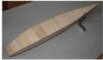
24: Sheet the underside of fuselage with 1/16" sheet, with the grain across the width of the fuselage. Also fit ply tailwheel mount.
