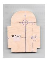
20: Drill holes in bulkhead for the motor, as shown, this was attached by bolts through the bulkhead directly into the motor. These holes are offset as shown, as I found that 2 degrees of right thrust was required. I used a wood spacer to pack between the motor and bulkhead to avoid changing the size and shape of the bulkhead.
