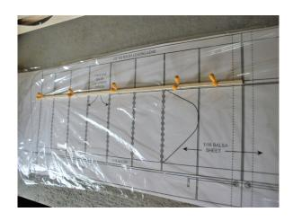
2: Glue in all ribs, and use the template to ensure correct angle of centre rib.
