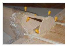
30: Now, with yet more cling film in front of F3 on the fuselage, fit the other F3 and adjust to size as necessary. Fit F2, the 1/4sq top spine and some additional 1/4sq on the wing deck, this is needed to have something to glue the sheeting to. Then, as for the rear decking, make a card template and then cut and add 1/16 sheeting.
