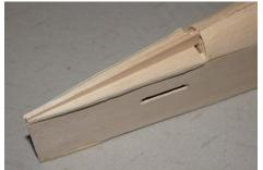
26: The next job is to make the infill between the horizontal and vertical stabilisers. To do this, I made a t-piece from the stabiliser sheet offcuts and tack glued lightly in place on the fuselage. Then, again, tack glue some scraps for the infill, this is now easy to sand to shape. When done, remove from fuselage and take out the t-piece, leaving two perfect shaped infills.
