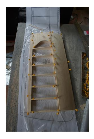
8:Glue sheets for the wing tips together and roughly sand to shape.
