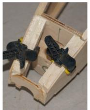
22: Fit some scraps of wood to the bottom of the nose to allow for shaping.
