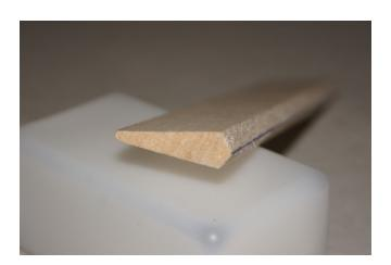
13: Cut ailerons to size and draw a line down the middle of the front edge and shape as shown in picture.
